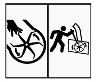
Never use your hands to clear a clogged auger. Never allow anyone to reach into the chute, force objects (i.e. bars, poles, etc.) down the chute, or otherwise come in contact with a rotating fan or with a non-rotating clogged fan or auger. Never allow anyone to reach into the chain drive housing. The auger can crush and/or dismember. Keep everyone clear of the auger until the prime mover engine is off and the hydraulic pressure has been relieved.
